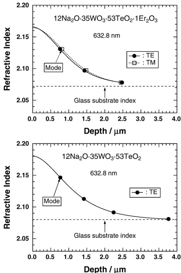
Fig. 2. Refractive-index profiles of  $12\text{Na}_2\text{O}\cdot 35\text{WO}_3\cdot 53\text{TeO}_2\cdot 1\text{Er}_2\text{O}_3$  glass waveguide for TE and TM modes (top) and of  $12\text{Na}_2\text{O}\cdot 35\text{WO}_3\cdot 53\text{TeO}_2$  glass waveguide for TE mode (bottom) at 632.8 nm.
