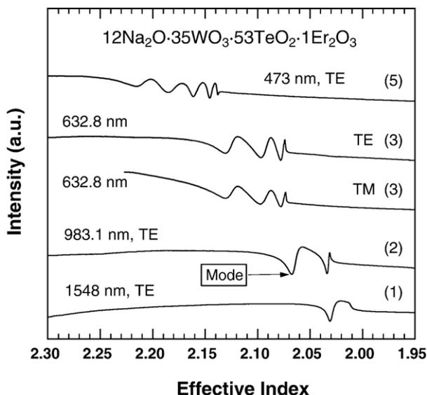
Fig. 1. Waveguide modes of ion-exchanged  $12\text{Na}_2\text{O}\cdot 35\text{WO}_3\cdot 53\text{TeO}_2\cdot 1\text{Er}_2\text{O}_3$  glass at 473, 983.1 and 1548 nm for TE mode and at 632.8 nm for TE and TM modes.
